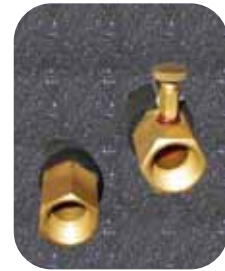
Completed With Internal Thread Chilled Water Header
